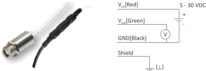
Fig. 6.2: Terminal assignment voltage output (mV)
