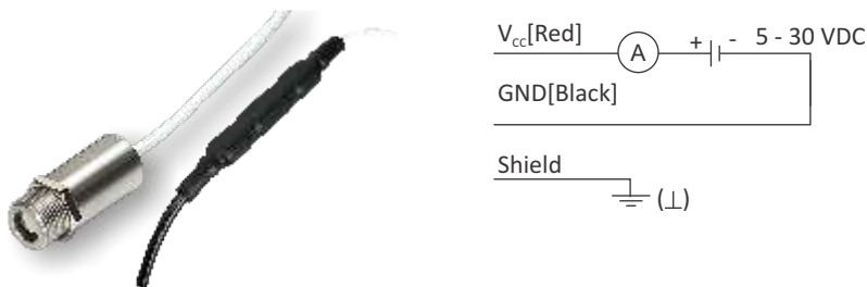
Fig. 6.3: Pin assignment current output as two-wire sensor
