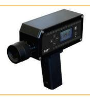
P390 is specially designed portable IR Pyrometer for non-contact temperature measurement of metallic surfaces and in flame heated furnaces i.e through flames and flue gas. At a wavelength of 3.9um, hot furnaces gases and clean burning gas flames are quite transparent and therefore permit temperature measurement of substances to be measured.
