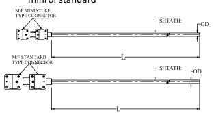
With this type the plug is directly connected to the metal sheathed thermocouple, mini plug for T/C dia  $\leq$  1.6 mm or standard plug. The contacts are made of compensating conductor, the outer body of temperature resistant plastic material. The maximum plug temperature is 150 °C. Plug and coupling are put together polarity-correct and thus offer optimum contact reliability. Other plug systems are available on request, as well as suitable couplings. (Please specify when ordering.)
