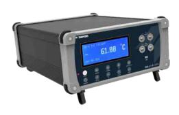
is essential. Two channel input provides A, B & A-B measurement on LCD Display. The device is providing exceptionally stable cold junction compensation with choices for user like Automatic, Off and External.
