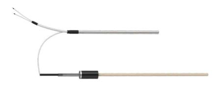
Tempsens offers special Reference thermocouples for high temperatures upto 1500°C for highly accurate temperature measurement. These Thermocouples are offered in platinum / Rhodium (type R, S or B) elements with a high purity Alumina insulations and sheath materials.
