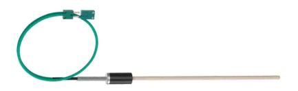
Tempsens offers special Reference thermocouples for high temperatures upto 1500°C for highly accurate temperature measurement. These Thermocouples are offered in platinum / Rhodium (type R, S or B) elements with a high purity Alumina insulations and sheath materials.
