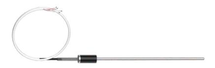
High accuracy Platinum Resistance Thermometer (PRT) is an interpolating instrument converting temperature to resistance. It works together with readout device to measure temperature or change of temperature. It has wide applications for dry-wells or temperature baths.
