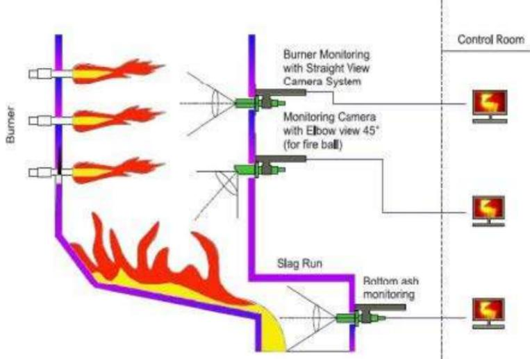
The High Temperature Monitoring System is the most cost effective solution for monitoring of fire ball in Boilers. Moreover it requires minimum maintenance from the operator part to run the equipment. Also water cooling helps to reduce the cost of Air Consumption. Only one analog signal cable required from site Control Panel to CCR.
