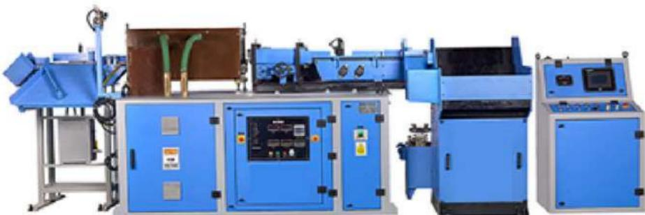
Induction heating is a non-contact process which uses the principle of electromagnetic induction to produce heat in a workpiece/object. When a conductive material placed into a strong alternating magnetic field, electric current flow in the material, and cause Heating.
