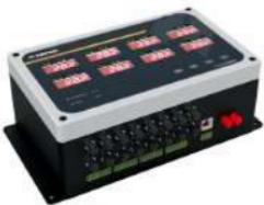
A fluorescence-based fiber optic monitoring system conducts real-time monitoring to accurately measure the temperature of the transformer's winding hotspot and switchgear contact points. It is a single-point temperature sensor. It is suitable for work in a harsh environment like high pressure, high temperature, and strong electromagnetism.
