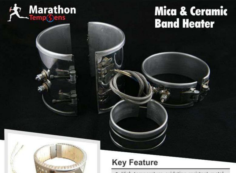
Mica & Ceramic Band Heaters offer efficient and economical heating solutions to pipes and tubes that require external indirect heating. These heaters are used to heat-up the external surface of drums or pipes for a gradual heat transfer. A mica core surrounds the precisely wound heating element, producing a thin, efficient heater.
