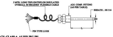
ACCURACY: CLASS-A, AS PER IEC-751 TEMP. RANGE: 0 TO 400°C RTD FOR PROCESS TEMP. MEASUREMENT
