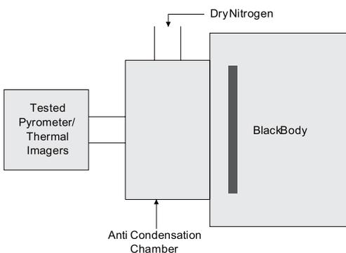
Along with LBBCH model tempsens blackbodies also offers anti condensation chamber around black body emitter for dry air/ nitrogen to prevent any ice build up or water vapor condensation in case black body operate below ambient. one end off the chamber will be fit to black body emitter and another hole of the chamber fits to optics of tested pyrometer or thermal imagers.
