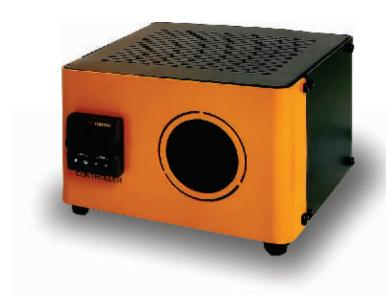
CAL FAST 400 BB offers medium temperature range from 50 to 400°C. It is a highly stable standered black body calibrator for calibrating non-contact type sensor like Pyrometer/IR Thermometers. The temperature of the calibrators is set and controlled by a self tuned PID controller with autometic super fine adjustment. in the double display the actual and set temperature values are soon. The BB cavity diameter is 50 mm with emissivity 0.97
