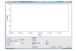
• CalSoft including for setting bath temperature and monitoring the PV. Graphical representations of PV/TIME with 2 hours data logging.
