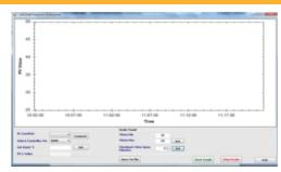
• CalSoft including for setting bath temperature and monitoring the PV. Graphical representations of PV/TIME with 2 hours data logging.
